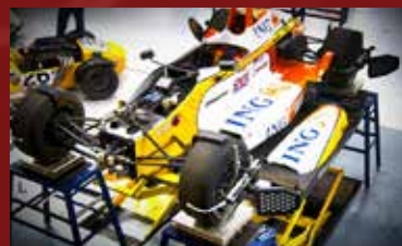
Wheel Alignment and Corner Weighting
